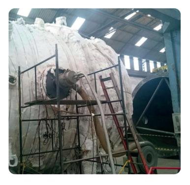
The heating system is a high velocity gas burner blowing hot air at velocity up to 260mph, the fuel would be LPG or Natural Gas and the burner can introduced in the nozzle of the vessel.
