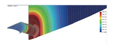
With the use of numerical modeling Tecnotrat makes available with the use of sophisticated finite element software to analyze the thermal cycle of heating, soaking and cooling through simulations with the application of heat flux representing the heating regions of the heat treatment in order to establish the best procedure to be used without generating harmful residual stresses on the equipment.
